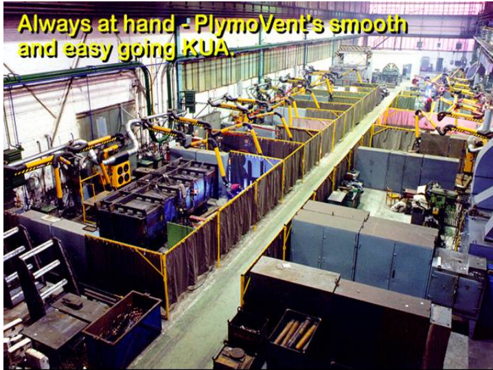
Figure 23. Articulated fume extraction arms with a built-in damper and a task light.
