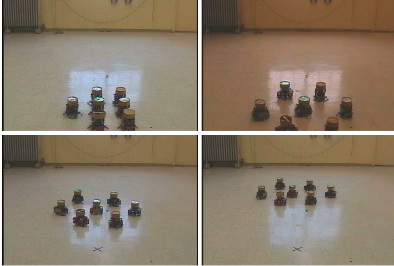
Fig. 6. Seven robots self-organize into a hexagonal formation, which then successfully moves towards a light source (a window, not the reflection of the window). Pictures taken at the initial conditions, at two minutes, fifteen minutes, and thirty minutes.
