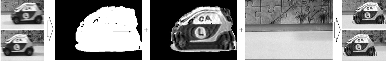
Figure 1. From two real blurred frames (left), we automatically and simultaneously estimate the motion region, the motion vector, and the image intensity of the foreground (middle). Based on this and the background intensity we reconstruct the two frames (right).
