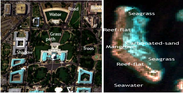
Figure 5 RGB composite of a) Washington DC and b) Enrique Reef images, showing also their ground truth.
