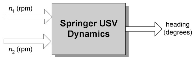
Figure 6: Block diagram representation of a two-input USV
