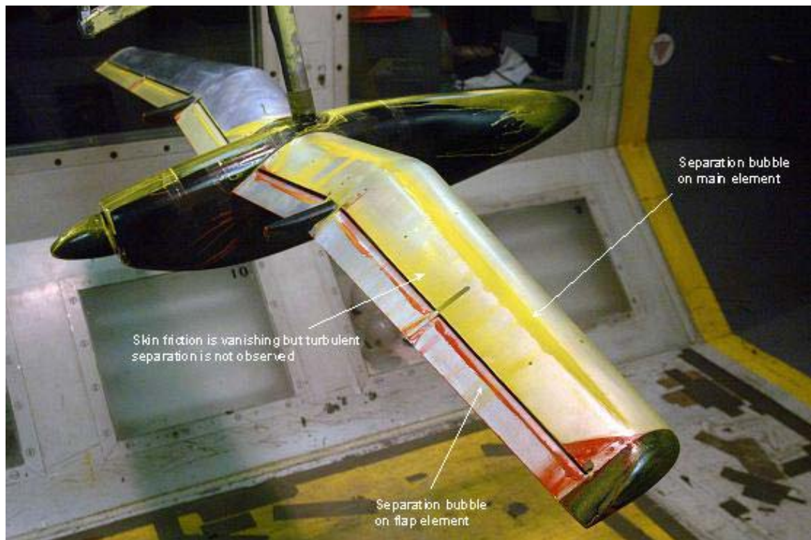
Figure 17: Oil flow visualization
