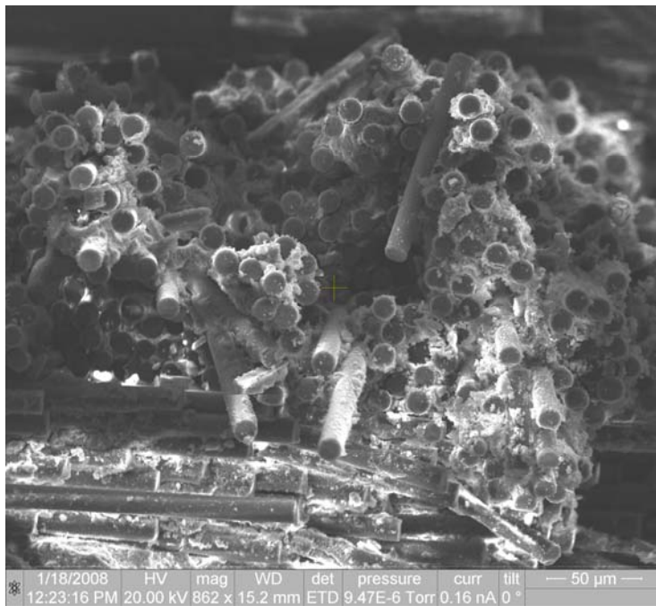
Figure 60. Specimen CG-11 (1200°C, air, 73 MPa, 100 h), 862X.
