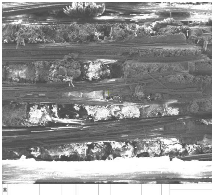
Figure 56. Specimen CG-11 (1200°C, air, 73 MPa, 100 h), 108X.
