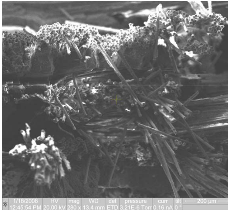
Figure 57. Specimen CG-11 (1200°C, air, 73 MPa, 100 h), 280X.
