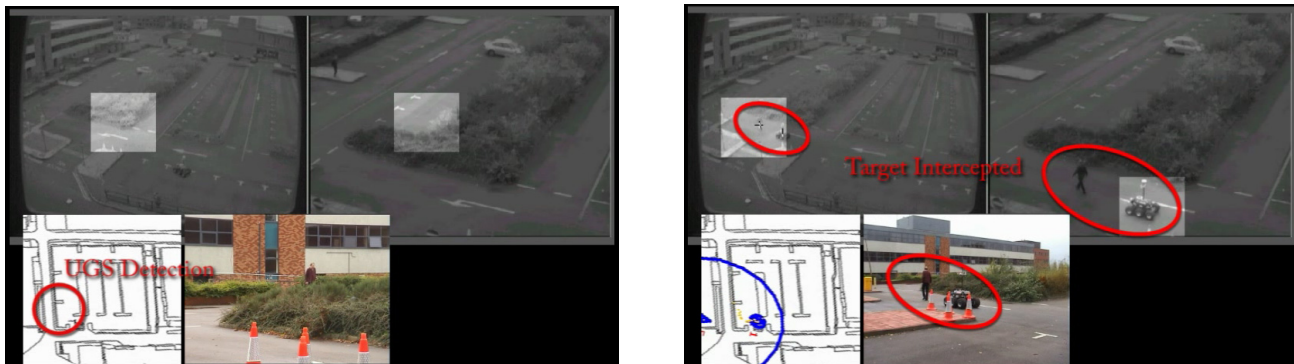
Figure 4: The UGS was used as a trip wire to cue the CCTV FOV; the latter are the light grey squares
