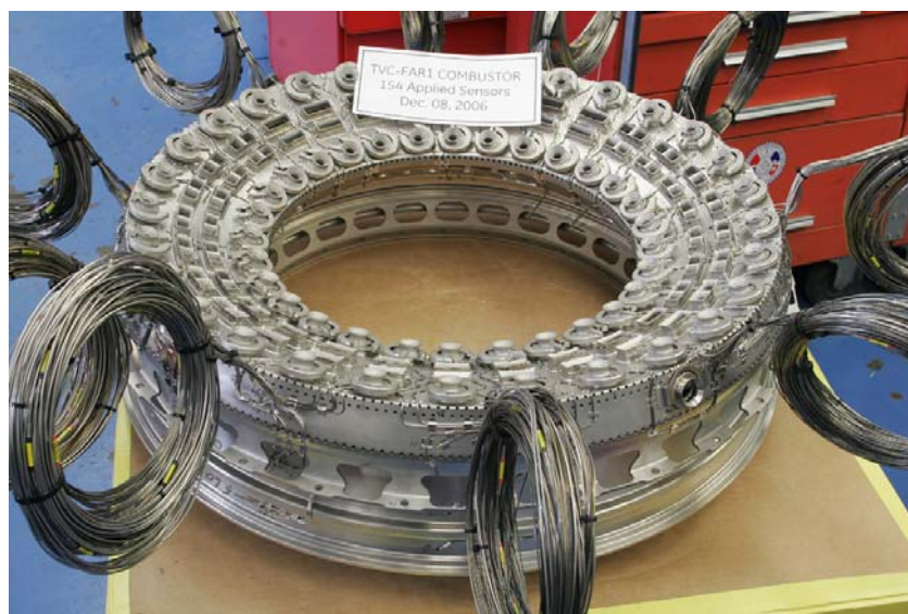
Figure-3: TVC Full Annular Rig (FAR) Hardware with Instrumentation
