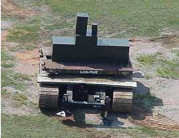
Fig. 3. The data collection setup showing target configuration 1 on turntable at 90° aspect (broadside).
