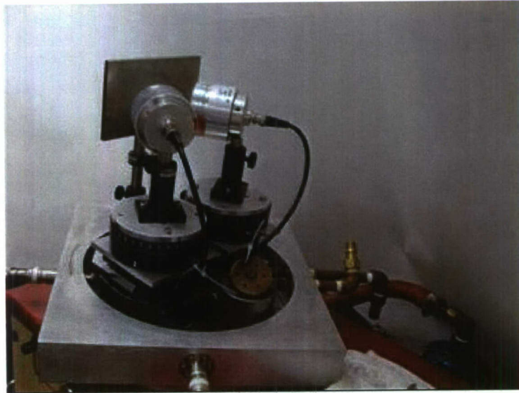
Fig. 3.2 Experimental setup for measurements of ultrasonic beam reflection.
