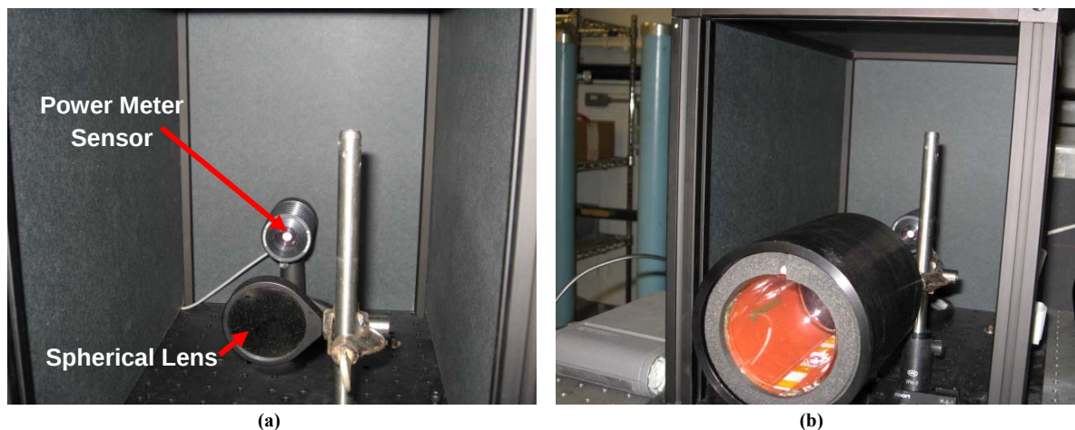
Figure 33. Pictures showing the power meter's sensor, spherical lens, and iodine filter mounted in a box with the front panel removed. The picture on the left (a) shows the sensor and the lens without the filter in place, and the picture on the right (b) shows the filter in place and ready for testing.
