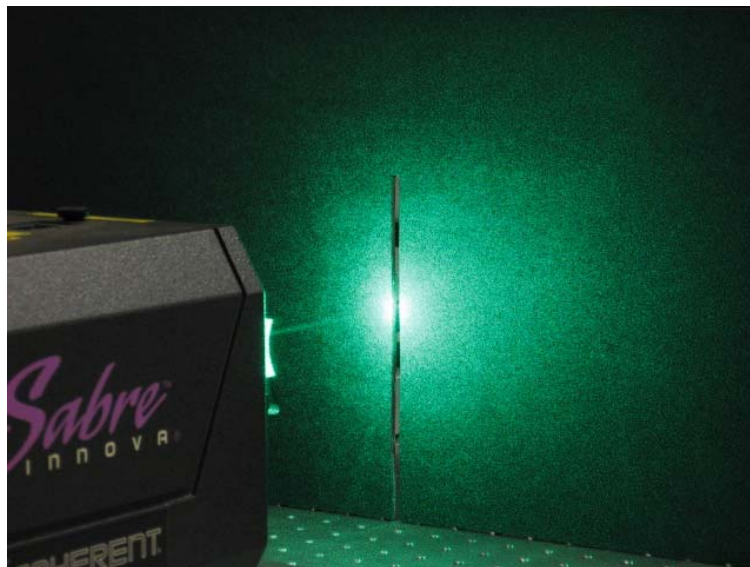
Figure 35. Picture showing one of the slotted boards used in the second experimental setup. Note the green glow that the board stops from further propagation while still allowing the incident laser beam to pass.
