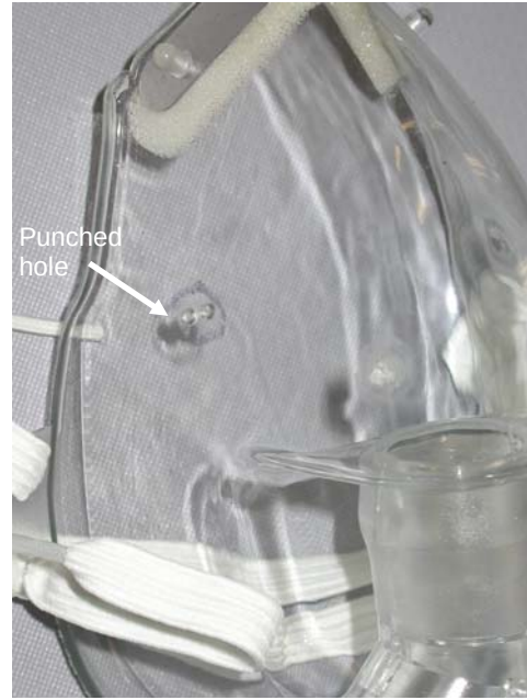
Figure 2: Holes in HiOx Mask for simulated leakage.
