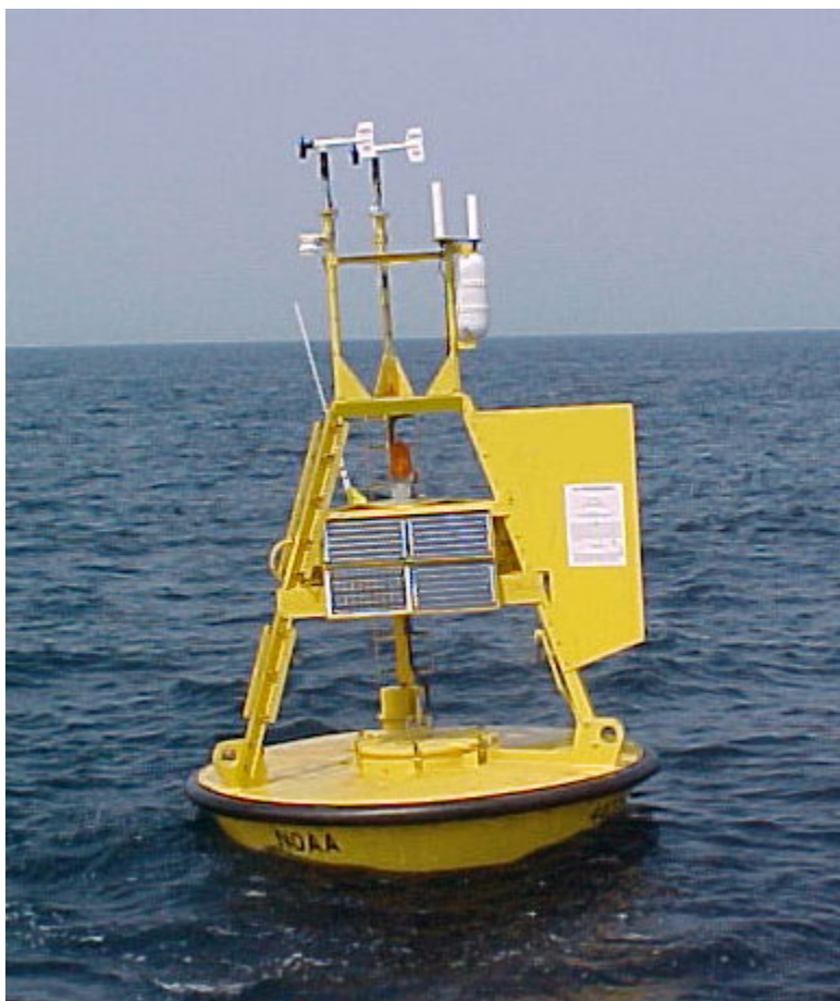
Figure 7. A 3 meter discus buoy, the type at Station 46131 Sentry Shoal
