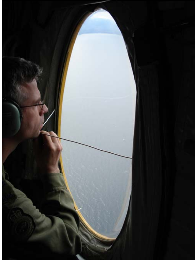
Figure 6 The wire apparatus used to control field of view
