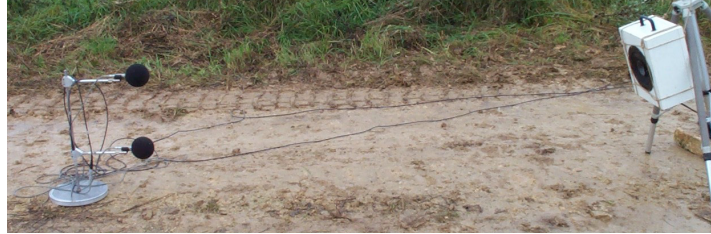
Figure 15: Device for the measurement of the road's acoustic resistivity
