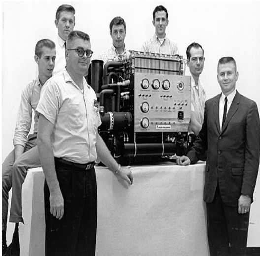
Figure 1 Allis Chalmers 5kVA Fuel Cell
