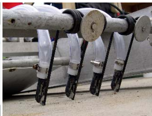
Figure 5. Spring-loaded seed injecting nozzles.
