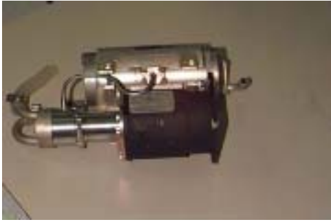
Fig. 7, Original 7050 compressor integrated in the dewar/FPA assembly.
