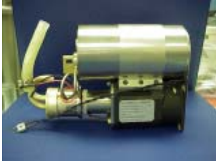
Fig. 8, US Army qualified OWL compressor integrated into the TISS dewar/FPA assembly.
