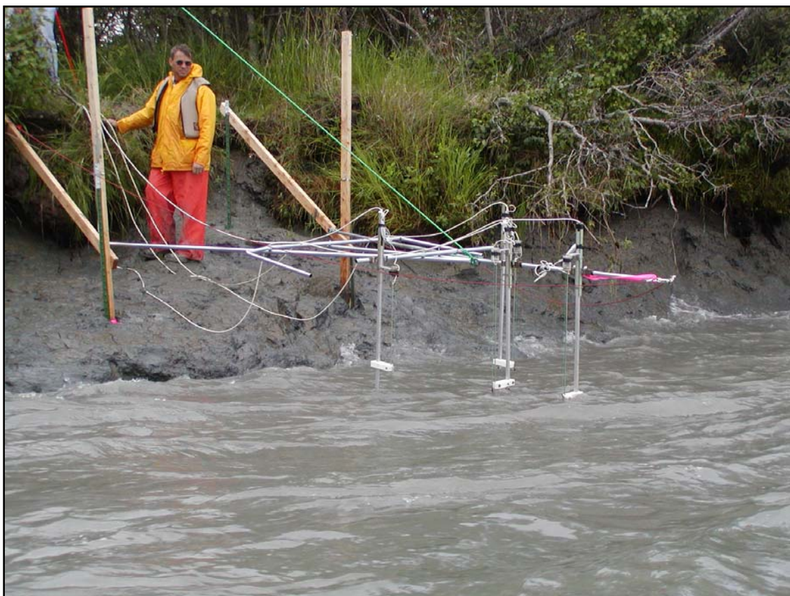
Figure 23. Wave stand supporting four wave rods used in wave measurements at RM 10.5. This site is on the left bank (looking downstream) about 0.5 mile upstream of Beaver Creek. Green rope used to raise and lower wave stand for installation, repair, and cleaning of gages as well as raising and lowering to deal with varying water level due to tides.
