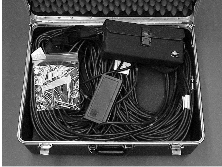
Figure 1. The USLM system is shown in the carrying case used for shipping and transporting the USLM system to and from the work site. The hand-held unit case (upper right), protective case for the hydrophone (middle), hydrophone cable, and adapters (in bag at left) are shown in the case. The wooden case containing the in-air microphone is located inside the hand-held unit case. The normal placement of the hand-held unit case is in the opening of the cable coils in the right-hand section of the case. The white tags are depth markings for use in placing the hydrophone on-site in the water.
