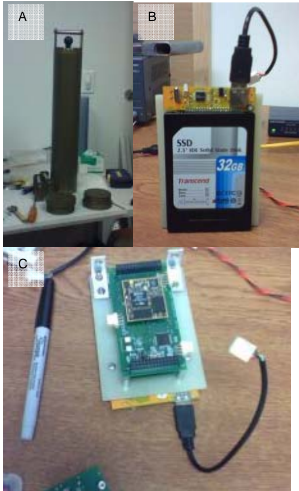
Figure A. A) Recorder external view. B) Front of the “guts” showing USB flash hard drive, which can be switched out easily as capacity increases. C) Back of the “guts” illustrating the small size of the processor.
