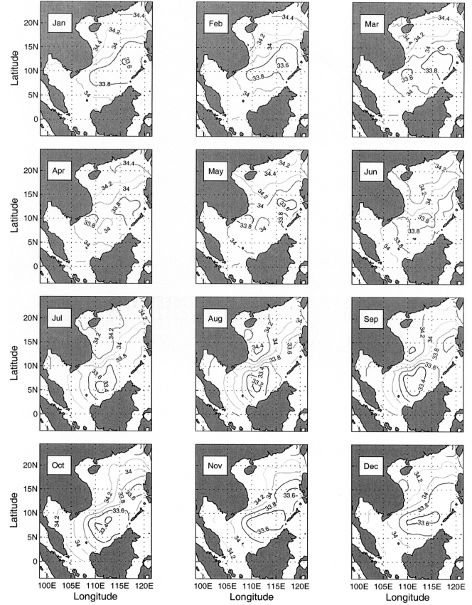
Fig. 8. Monthly mean salinity (ppt) field at 50 m depth with 0.02 ppt contour interval.
