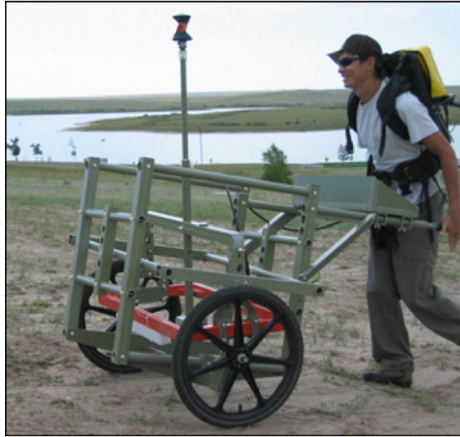
Figure 33. The gimbaled cart system was deployed over a test plot at the FLBGR GPO site.
