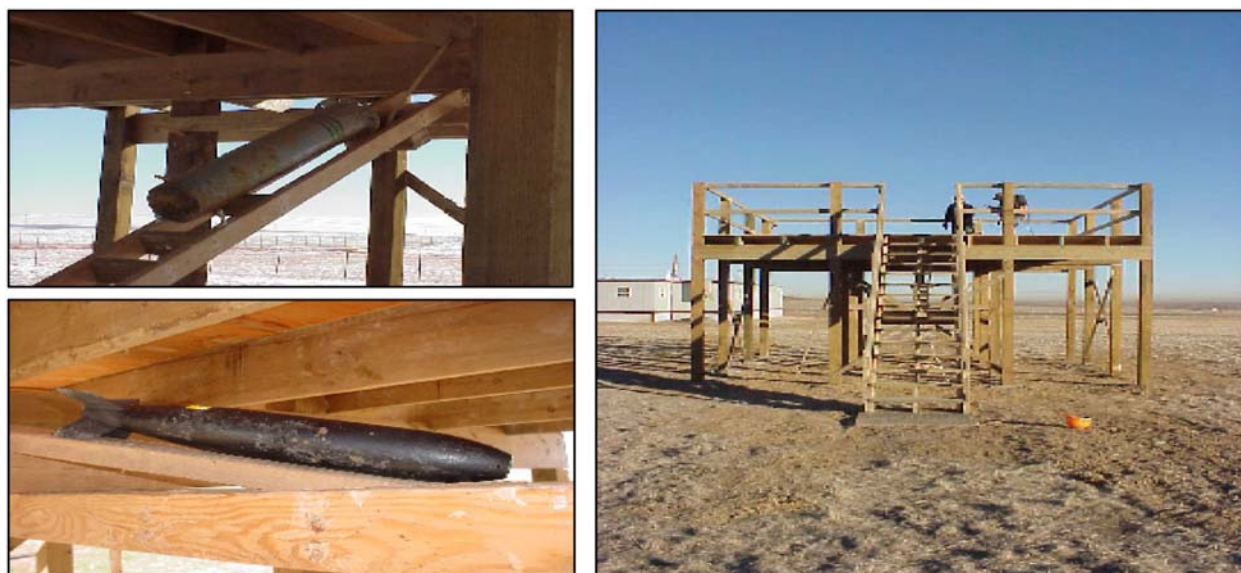
Figure 7. The platform was constructed to allow items to be geophysically characterized at sensor offset of up to 8 feet. Below the wooded platform floor was a jig used to house the test items at measured offsets and orientations. Signatures were collected from various UXO, non-UXO, and calibration items.
