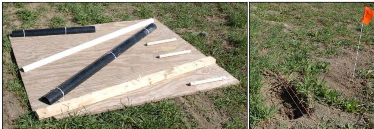
Figure 43. Ruts and stick mats used to simulate high micro-topographic changes on the Ashland Test Plot.
