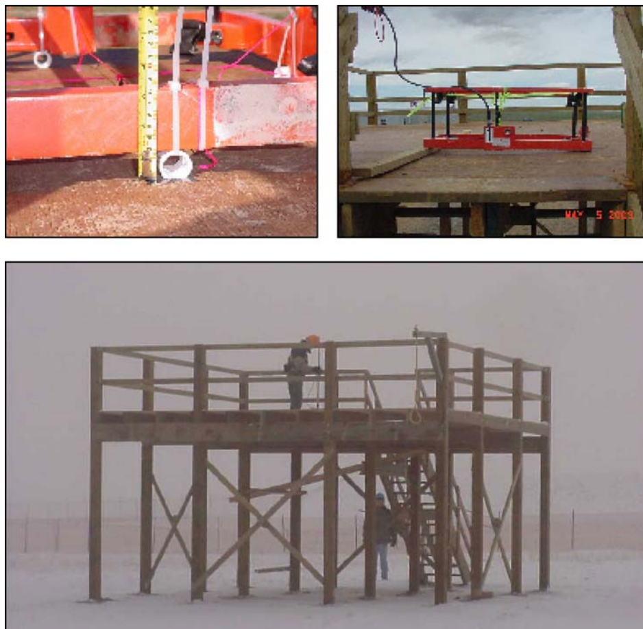
Figure 8. A non-metal platform was constructed at the FLBGR, in Denver Colorado. This platform was used to measure various geophysical signatures from UXO and non- UXO items.
