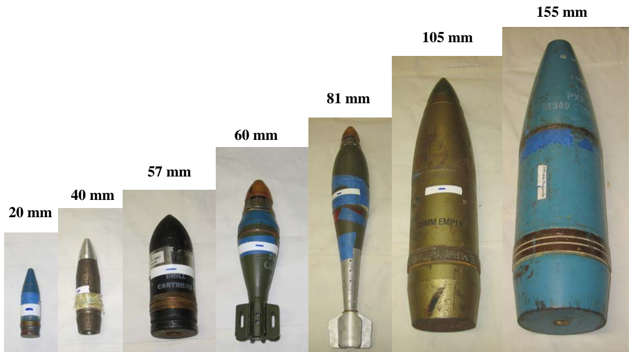
Figure 21. UXO targets used in the measurements of characterization standoff range.
