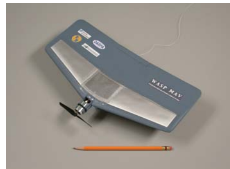
Figure 5: First generation DARPA Wasp micro-air vehicle showing custom batteries (silver quadrilaterals, top and bottom) integrated as wing-skin at the leading-outboard-edges.
