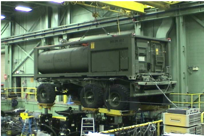
Figure 7 Experimental setup consisting of a PLS trailer carrying a "Hippo" tank module mounted on an n-post motion simulator and instrumented to measure the tire and suspension system deflection time-histories.
