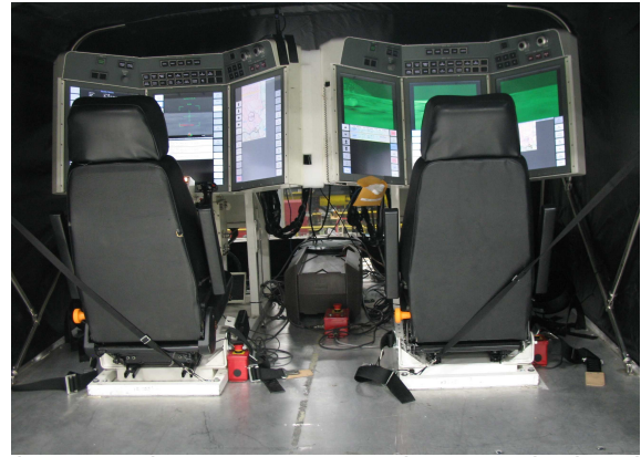
Figure 5. (left) TMBS with crewstation platform, enclosure and two CAT crewstations attached and (right) two CAT crewstations on the crewstation platform.
