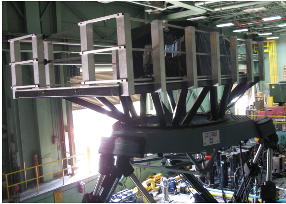
Figure 5. (left) TMBS with crewstation platform, enclosure and two CAT crewstations attached and (right) two CAT crewstations on the crewstation platform.
