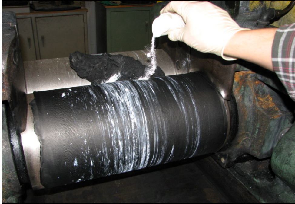
Figure 4. Nitrile rubber compound being produced on rolling mill.
