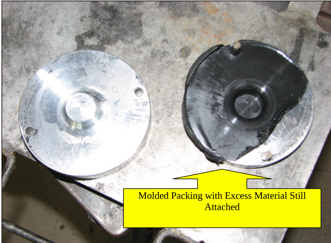
Figure 8. Finished packing after pressing with excess material still attached.
