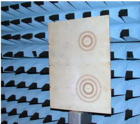
Figure 3: Panel with six antennas located in a square grid
