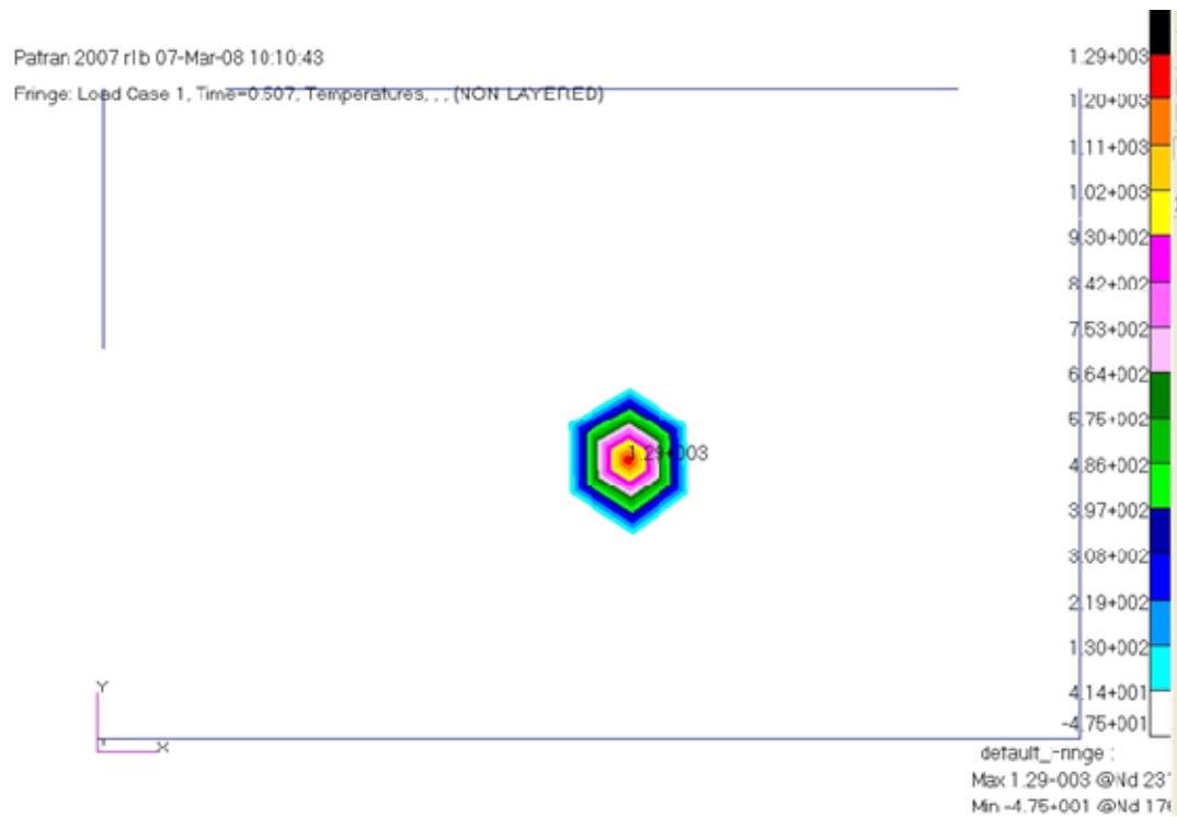
Figure 46. Temperature gradient across a 3d aluminum plate at t = 0.5 sec.
