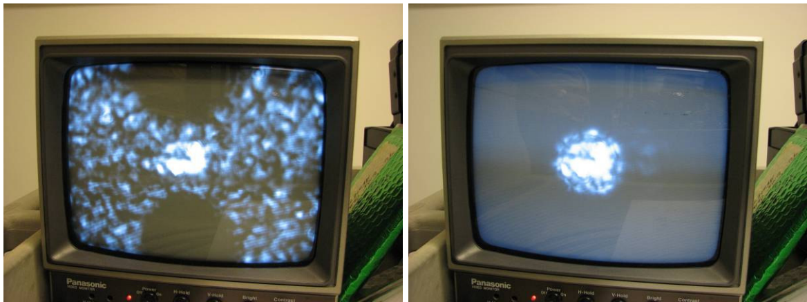
Figure 23: Camera Aided Alignment: Entire Output (left), Core Output (right)
