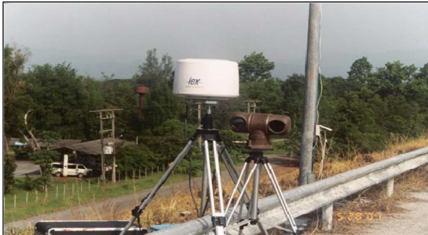
Figure V-5. Screen Shot of ICX ground radar from www.ICX.com used for tracking ground targets at Fort Hunter Liggett 2007 field exercise and Thailand demonstration.
