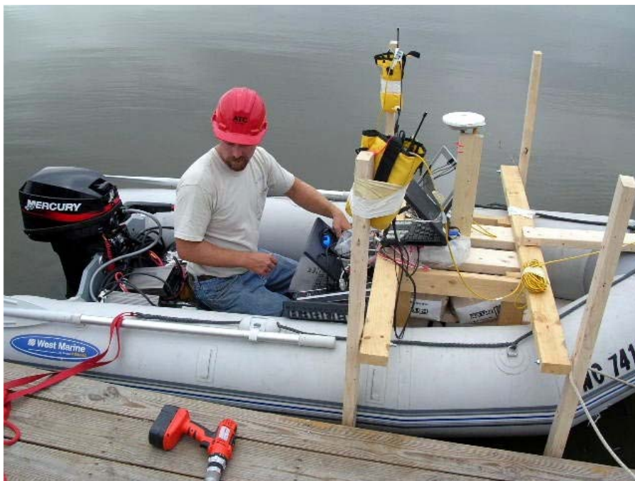
Figure 6. GEM-3 platform used to survey the littoral region.
