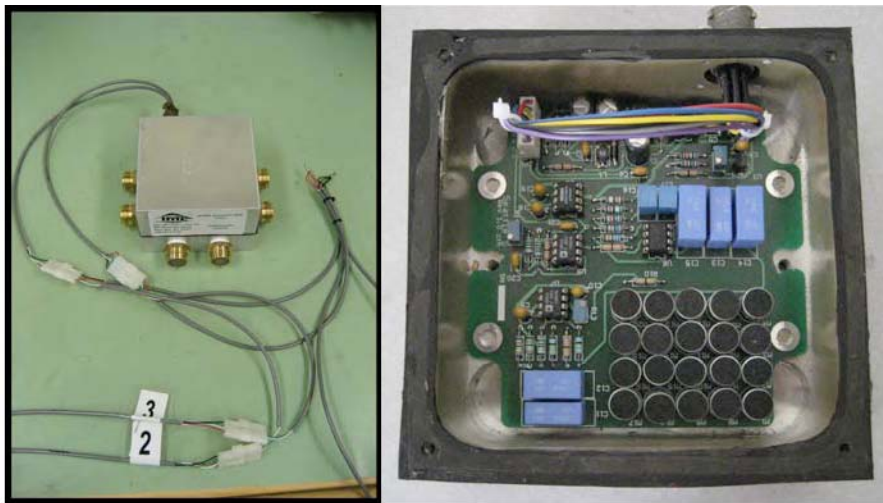
Figure 17: The IML infrasound gauge is pictured above. The exterior view is illustrated to the left with six of the eight ports for hose connections. The interior view of the gauge is illustrated to the right with the 20 microphone cartridges in the lower right and the accompanying signal conditioning and filtering electronics.
