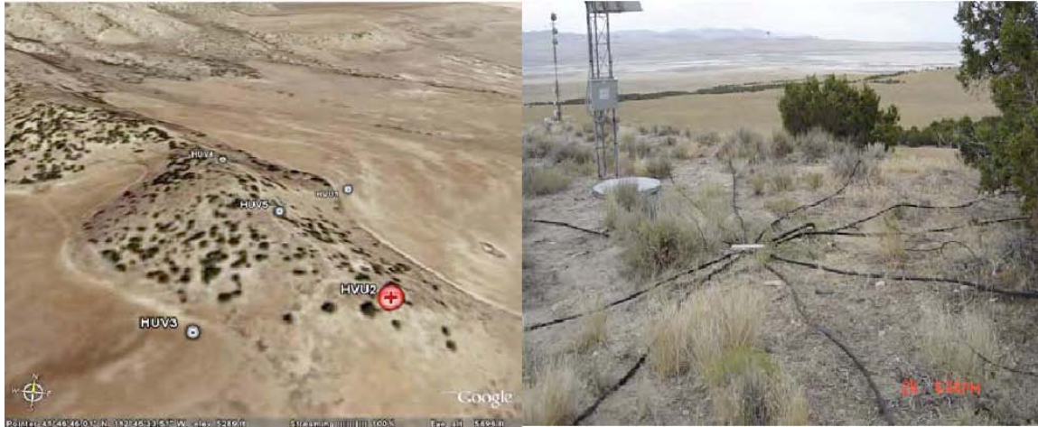
Figure 6: Infrasound array configuration at HVU (left) and one of the sensors attached to a set of porous hoses (right).
