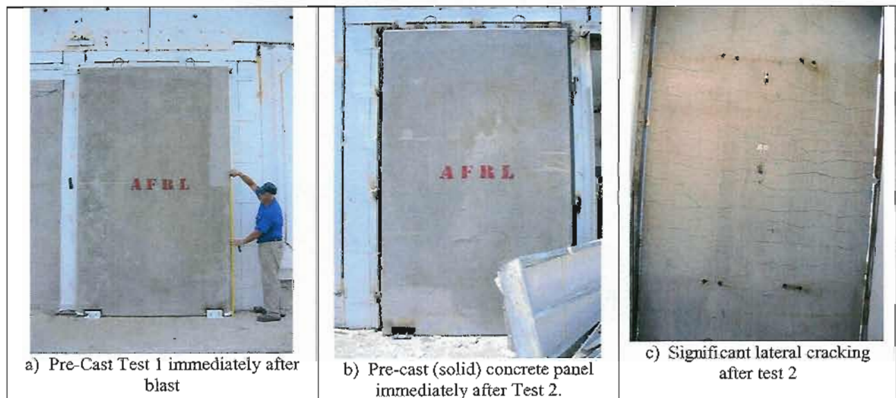
Figure 8. Post test photos of the precast concrete panels
