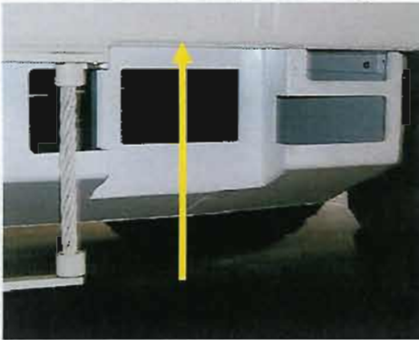
Front & Aft End Sleeper Shoring Placement
