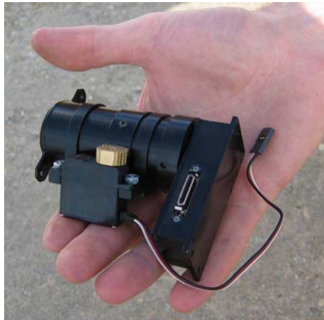
FIG 16 Assembled zoom system utilizing tunable GRIN lenses.
