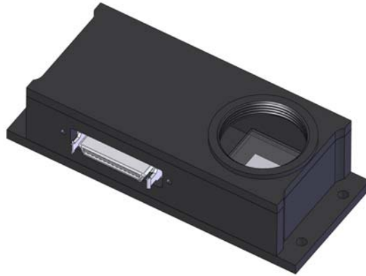
FIG 2 Sensors Unlimited SU-320us 1.7RT SWIR microcamera
