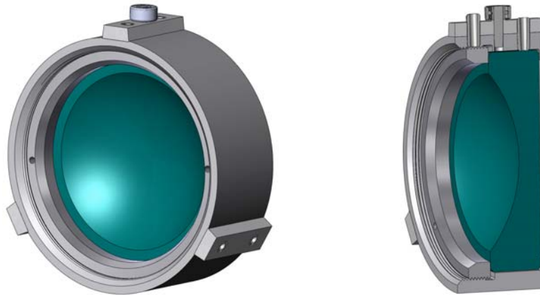
FIG 21 Isometric rendering and cross section of prototype 3.4 mount for lens 1.
