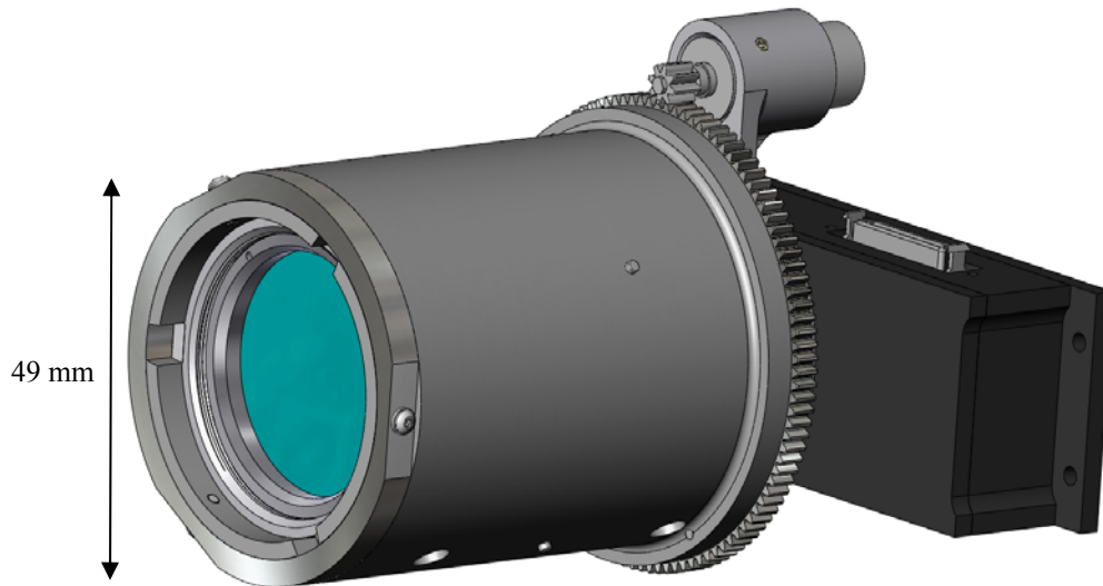
FIG 17 SolidWorks rendering of prototype 3.4 with SWIR camera.
