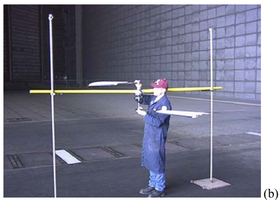
Fig. 12 – Mars Coaxial Rotor Hover Test; (a) conceptual sketch; (b) early stages of test hardware development
