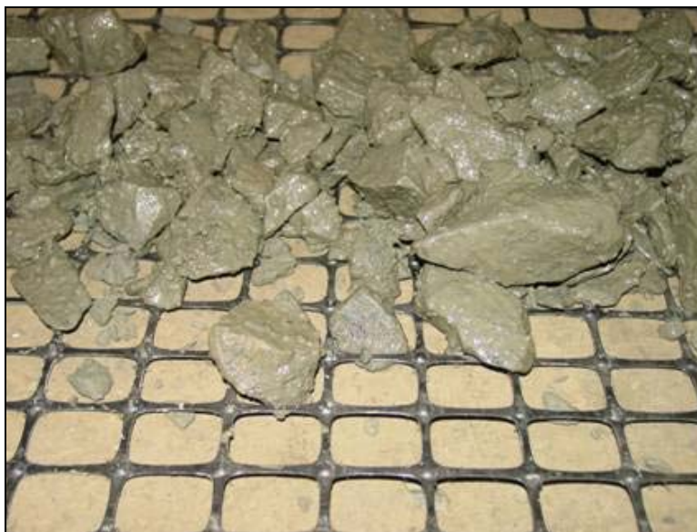
Figure 25. Close-up of geogrid and base aggregate particles.
