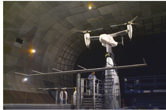
Fig. 5 – Full-Span TRAM Installation in the NFAC 40-by-80 Foot Wind Tunnel
