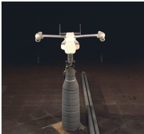
Fig. 22 – Full-Span TRAM in Airplane-Mode (Rotors Off)
