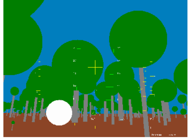
Figure 1: The screenshot of the 3-D simulated environment used for the experiments. The white sphere marks the target and dark gray (green) spheres with light gray cylinders mark the obstacles (trees).
