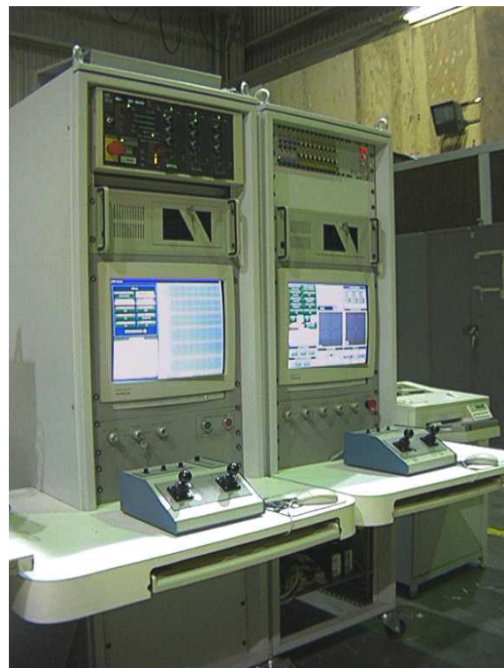
Figure 4. LRTA Primary and Dynamic Control Consoles.
