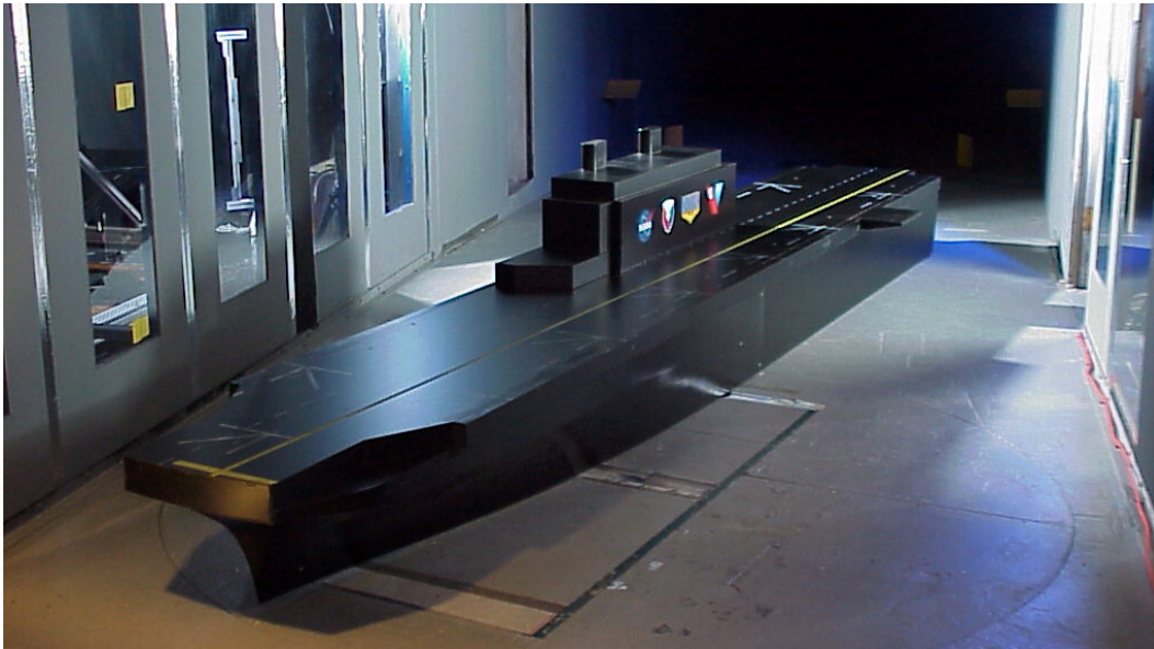
Figure 1. 1/48 th -scale amphibious assault ship installed in 7- by 10-Foot Wind Tunnel at NASA Ames.
