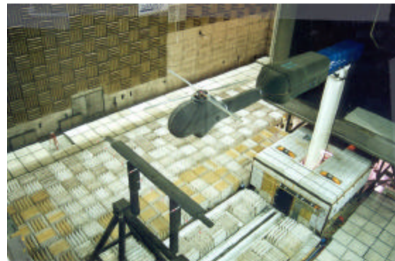
Fig. 1 BO-105 model rotor in the DNW
