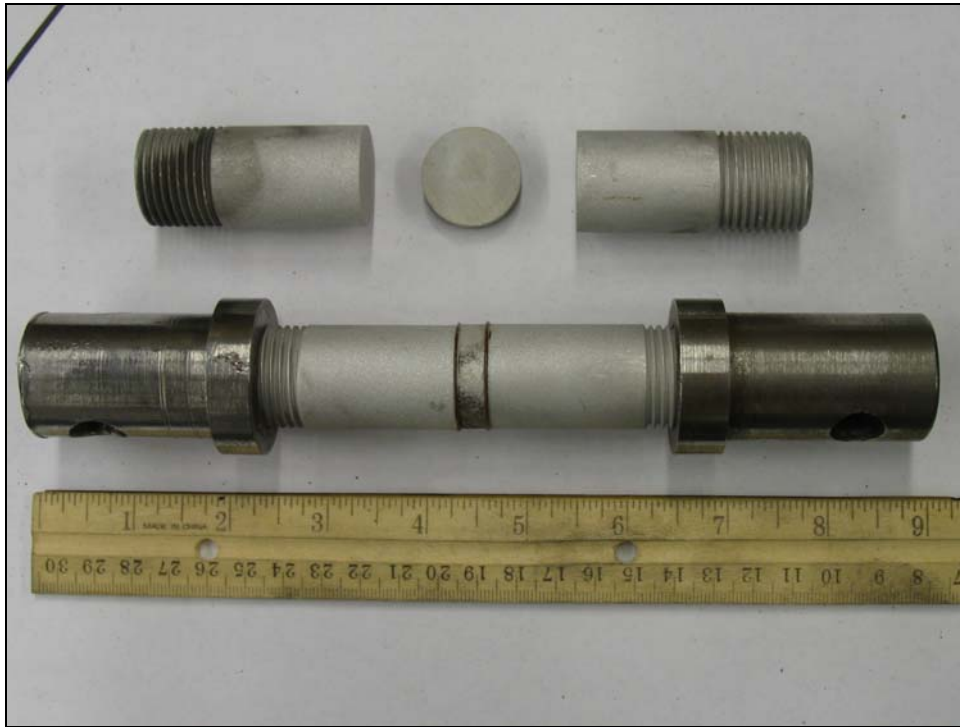
Figure 6. Bond bar adhesion test configuration.
