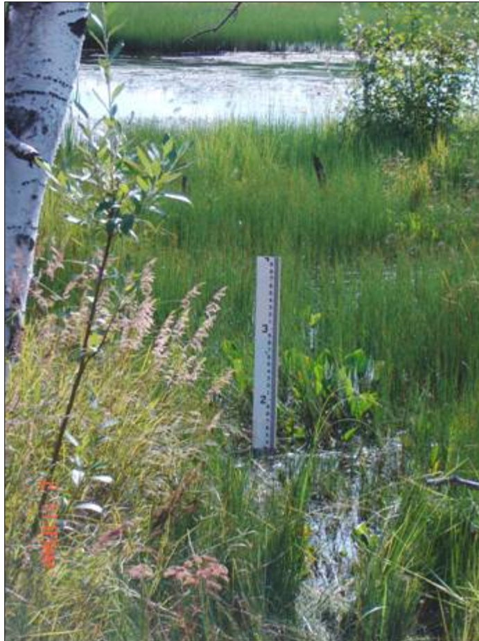
Figure 25. Staff gauge at Willow Creek Fen station for daily (May–September) water level measurement and posting with a web camera.
