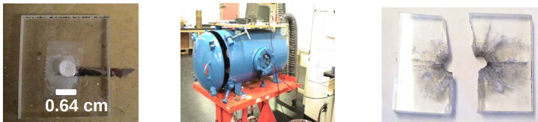
Figure 18. The photo on the top left is a Plexiglas plate with lead azide powder hand tamped in a hole in the middle. At the bottom of the plate is a nanolaminate foil strip that was in contact with the lead azide. The experiment test setup was put in a detonation chamber at Picatinny, shown above in the middle photo. The nanolaminate was ignited using a Nichrome hot wire. The reacting nanolaminate resulted in the detonation of the lead azide and shattering of the Plexiglas plate shown in the photo to the left.
