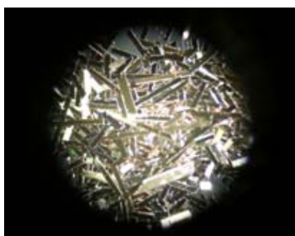
Figure 7. Photos summarizing the process of reduction of multilayer thin films to powdered material. Top left sheet a) is cut using the precision shear press b) into long fine thin strips of material (~2-10 cm long) which is then repeatedly passed through the shear press to produce an energetic multilayer powder d).
