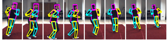
Figure 7. Multi-view Tracking. Tracking performance on the Jog sequence of subject S3 from HUMANEVA dataset; 250 particles are used for tracking. Illustrated is the projection of the tracked model into one of the 3 views used for inference.
