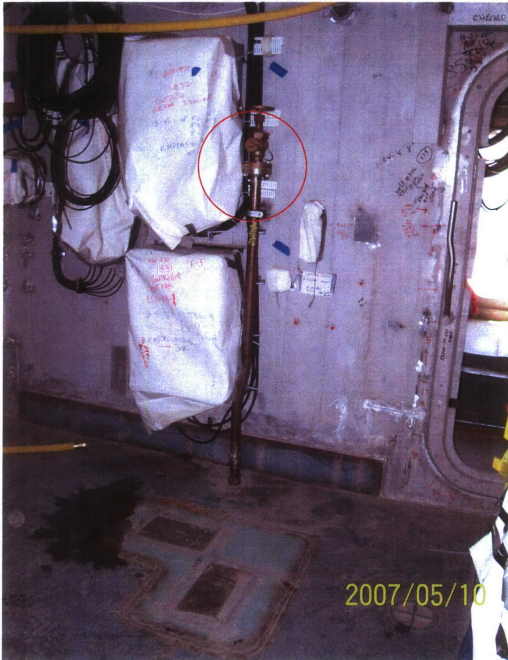
FIGURE 10. PORT AFT Saltwater Discharge with Mission Module Corner Pad on Deck. Tight clearance between discharge and module will likely cause hose to kink when charged.
