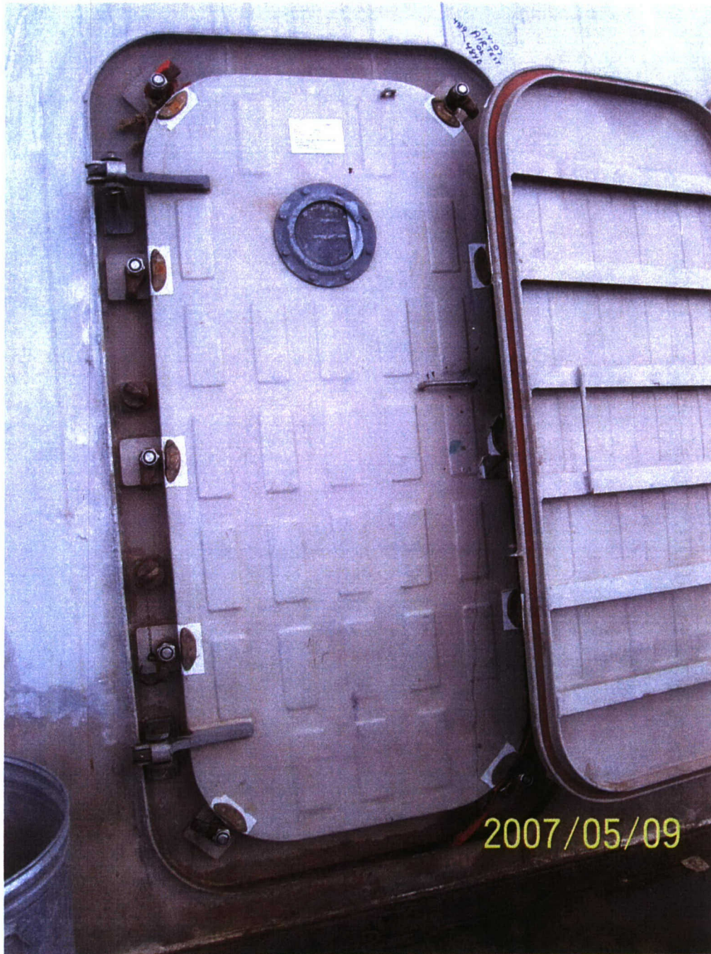
FIGURE 14. PORT Flight Deck Access Door is Blocked by Open Fuel Station Door.
