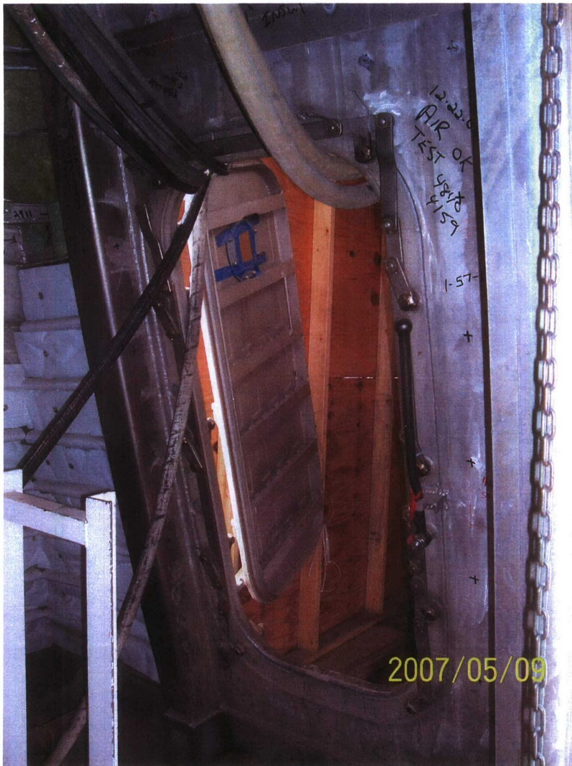
FIGURE 4. TRIGON Operating Console Obstructing Flight Deck Access Door.
