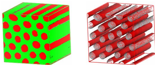
Figure 6. Mesoscale structures of bulk SIBS (PS phase is red, PI phase is green). The right site does not show PI phase for clarity.
